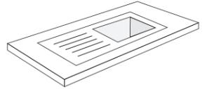
**minerva®** sink modules are made from a solid piece of material, the recessed sections may have a slightly different pattern on some décors due to the spread of the coloured chips.
