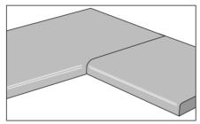
Using the isopropyl alcohol wipe supplied in the jointing kit, clean the cut edges of the worksurface. Ensure all surfaces are clean, dry and free of debris and dirt including the surrounding areas before proceeding to the next stage
