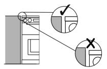
If the installation incorporates an Aga or other heat storage range, we would recommend a minimum of 60mm clearance needs to be allowed from the edge of the cooker to the worksurface.
